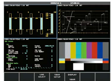
Multi Display Of 5 Bar, Waveform, Status, Picture (Ex, LV58SER01A 1 set is installed)
