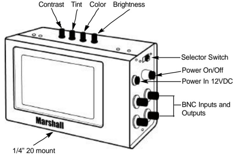
The **V-LCD4-PRO-L** is equipped with an active loop-through circuit. **This loop-through will only work when power is supplied to the monitor.** The monitor also has a 1/4-20 mount located on the bottom of the unit. This is useful when mounting the monitor on the top of a camera by using a hot shoe mount (Marshall part# **V-LCD-MT**) or other mounting devices.
