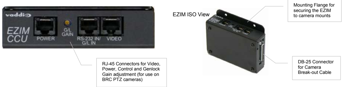
Figure 3: EZCamera Interface Module CCU (EZIM) with three (3) RJ-45 connectors for POWER, RS-232 IN / GEN LOCK and VIDEO (HD or SD), Top View (left) and Isometric View (right)
